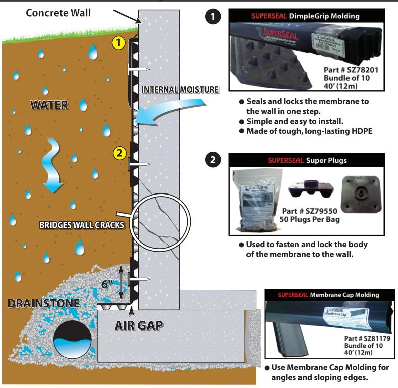
When installing on a poured concrete foundation, use DimpleGrip Molding for the top and side edges and Super Plugs to fasten the body of the membrane to the wall. Use Membrane cap molding for angles or sloping areas. Fasten with  $1 \frac{1}{4}$  or  $1\frac{1}{2}$  concrete nails. Use standard tar based caulking for seams or overlaps.
