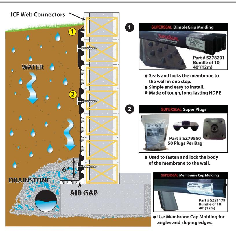
When installing SUPERSEAL Dimpled Membrane on an ICF foundation, always use DimpleGrip Molding for the top and side edges and Super Plugs to fasten the body of the membrane to the wall.
