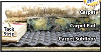
dimple design with dimples on the top and the bottom of the membrane providing 2 air spaces. These 2 air spaces allow the floor base and carpet pad to breathe independently. Keeping moisture out significantly increases the life of the carpet pad and carpet.
